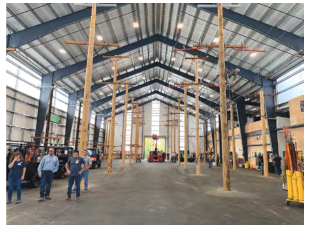
Local 659's line construction work is in demand, and the newly opened Northwest Line JATC's facility includes an indoor pole yard for training.
